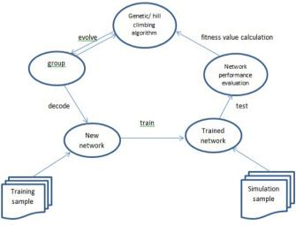
Figure 1. Structure of genetic and HC algorithms with neural network
