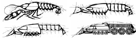
▲ Figure 5. Principles of the bionic forming in machine designing
