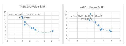
Pictures 7 and 8. The relation between heat transfer coefficient and response coefficient, in the houses of Yazd and Tabriz
