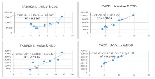
Figures 3 and 4 (above), 5 and 6 (bottom): the relation between heat transfer coefficient and CDD, HDD: Both charts in both cities indicate the existence of a relation between heat transfer coefficient and the maximum monthly Day temperature hot and cold in each of the 8 zone of the cities.
