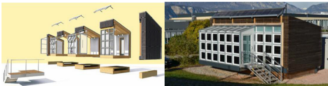
▲ Fig 6. The prototype connected residential unit in Trento, N. Italy (left) is organized in 3 modules and 2 side elements (right).
